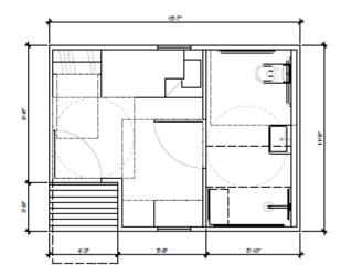
02 A2 - ADA UNIT PLAN A2.01 SCALE: 1/2" = 1'-0"
